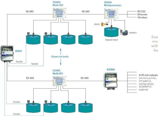
Example of three monitors individually monitoring and controlling nine tanks with two expansion modules to control feeders, lighting, and send data to a SCADA/PLC system.
