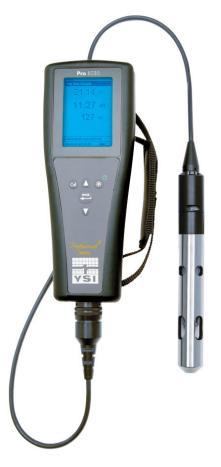
Parameters: pH ORP/Redox Conductivity Specific Conductance Salinity Total Dissolved Solids (TDS) Temperature
