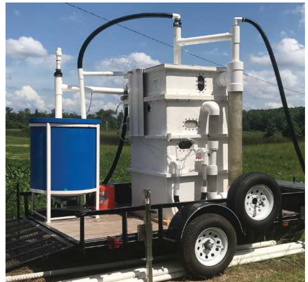
10 ft 3 Recirculating PolyGeysers unit, 1 hp regenerative blower, and linear air pump.
